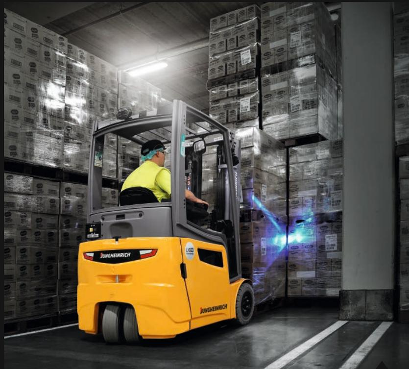
The Floor-Spot projects a blue light onto the floor in front of the truck, alerting employees to the approaching vehicle.
